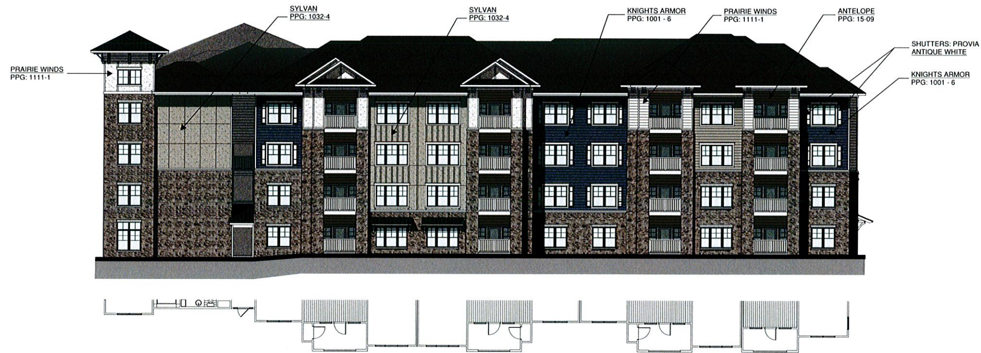
1 BUILDING TWO - EAST ELEVATION 3/32" = 1'-0" 0 4 8 16 32
