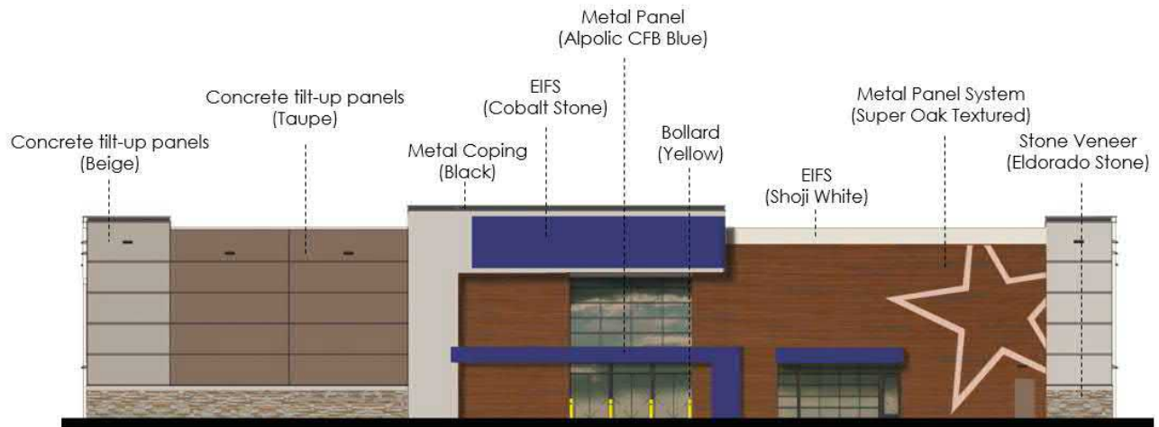
Figure 7: Recreational Facility – South Elevation
