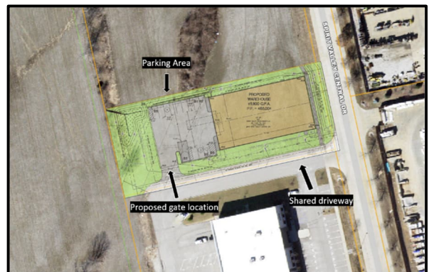
Figure 3: Circulation and access components
