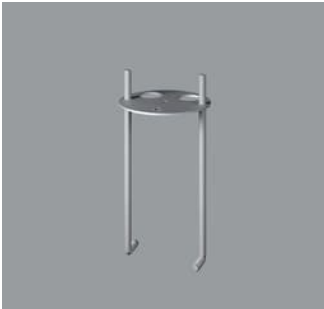
33979.000 Concrete anchor Mounting plate with threaded bar and fixing nuts M6. Individual parts to be assembled on-site. Weight 0.55lbs / 0.25kg
