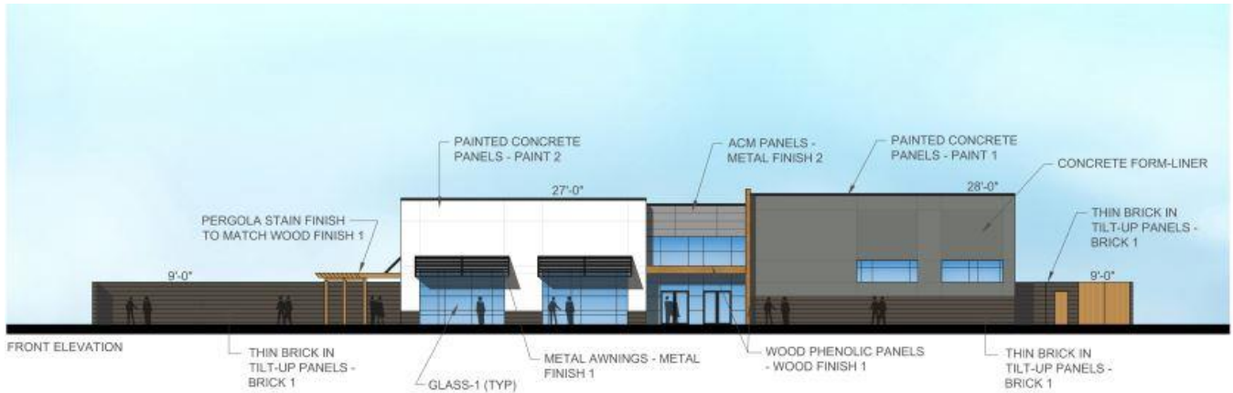
Figure 3: North side elevation
