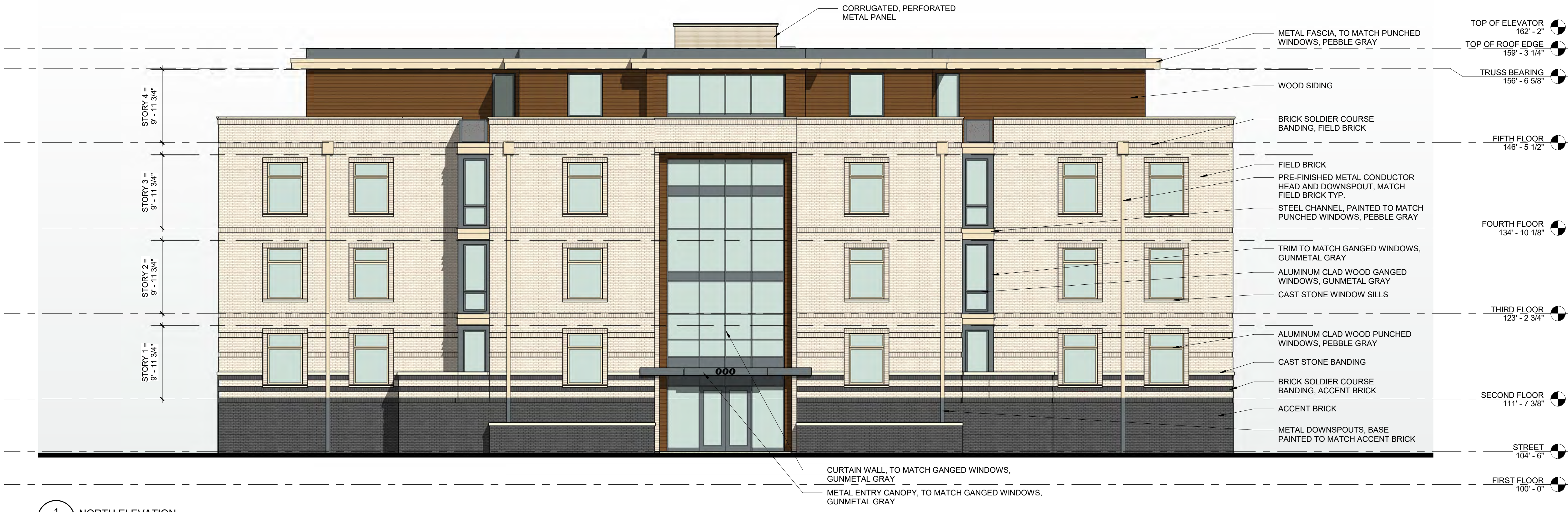
1 NORTH ELEVATION A.001 1/8" = 1'-0"
