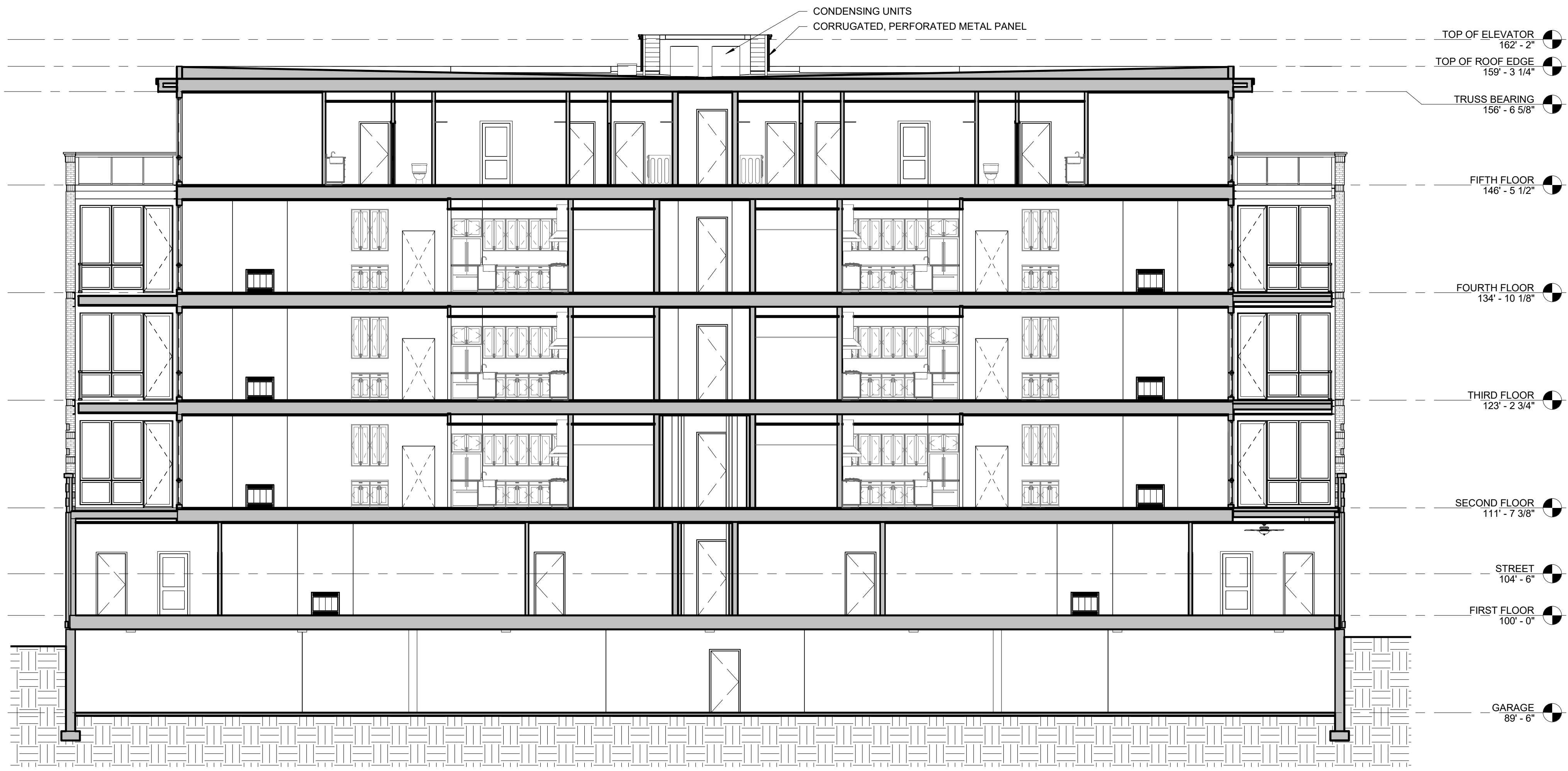
1 EAST-WEST BUILDING SECTION A.005 1/8" = 1'-0"
