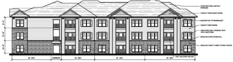
2 BUILDING TWO – EAST ELEVATION 3/32"=1'-0"
