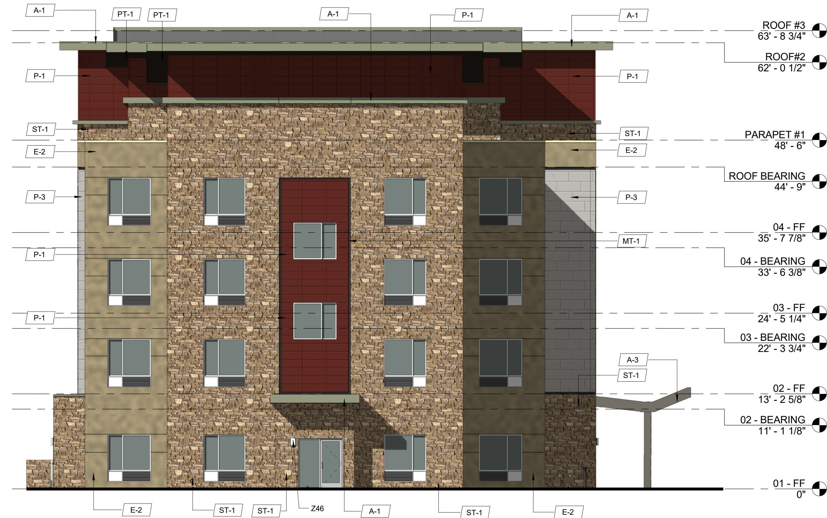
① WEST ELEVATION 1/8" = 1'-0"
