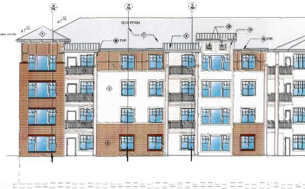
3 BUILDING D - INDEPENDENT LIVING - EXTERIOR ELEVATIONS SCALE: 1/8" = 1'-0"
