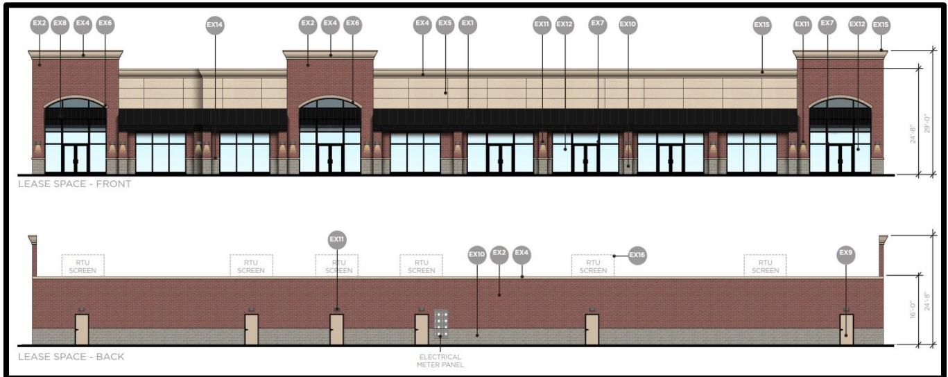
Figure 6: Retail building front and rear elevations
