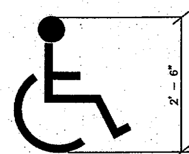
PAINTE GRAPHIC ON PAVING H.D.C.P. STALLS PAINTED BLUE HANDICAP SIGN (n.t.s.)
