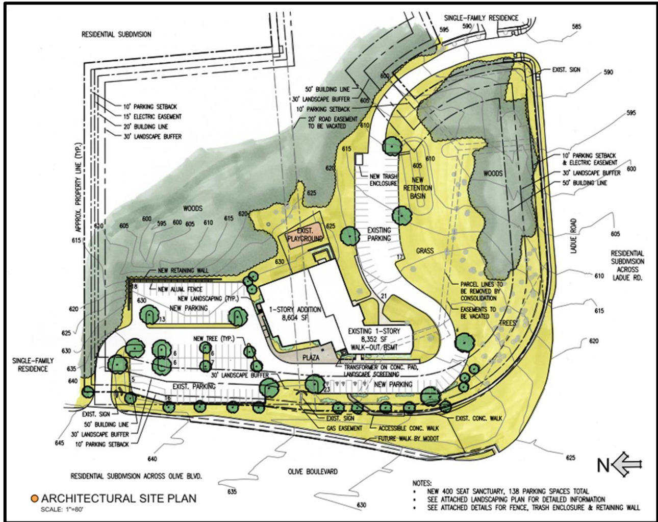
Figure 2: Color Site Development Section Plan
