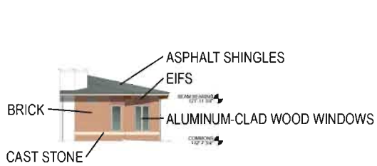
1 SOUTH ELEVATION - BUILDING B SCALE: 1" = 20'-0"
