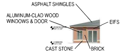
3 NORTH ELEVATION - BUILDING B SCALE: 1" = 20'-0"
