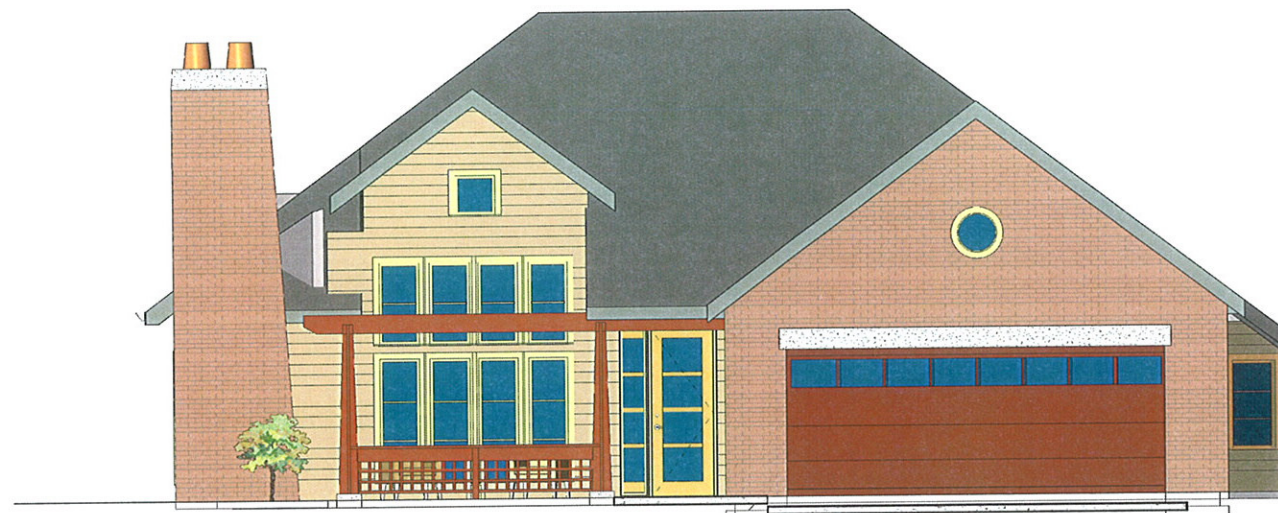
2 TYPICAL FRONT ELEVATION - UNIT C A20- 1/4" = 1'-0"
