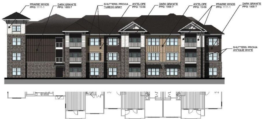
1 BUILDING TWO - EAST ELEVATION 3/32" = 1'-0"
