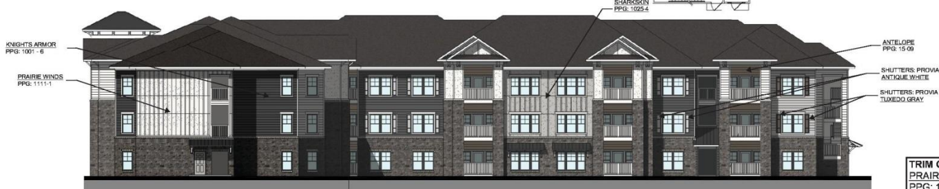
2 BUILDING ONE - NORTH ELEVATION 3/32" = 1'-0"
