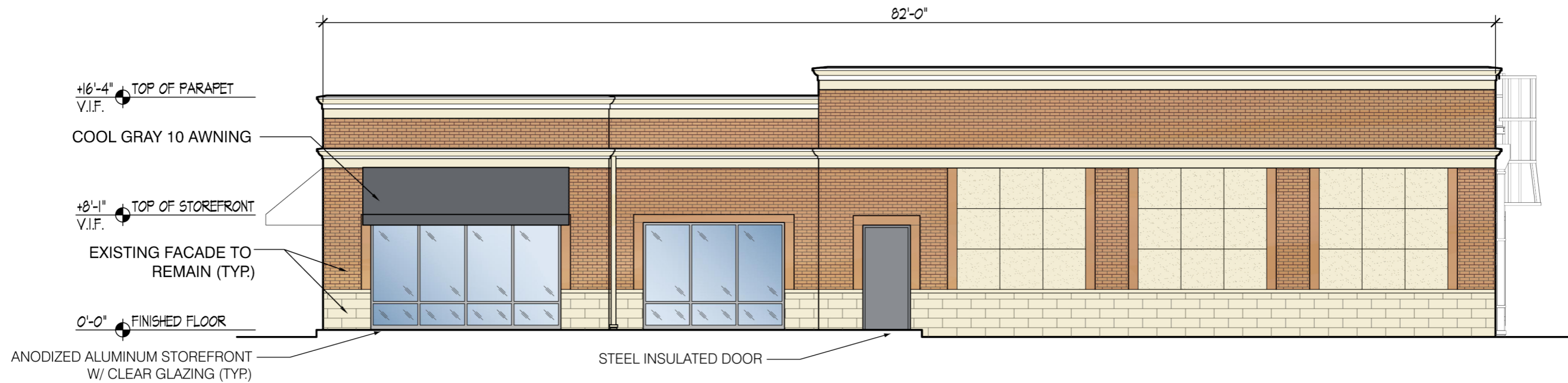
2 WEST ELEVATION - SIDE 1/8" = 1'-0"
