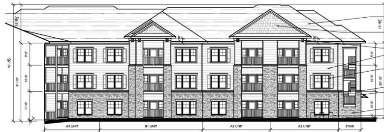
2 BUILDING THREE - WEST COURTYARD ELEVATION 3/32"=1'-0"
