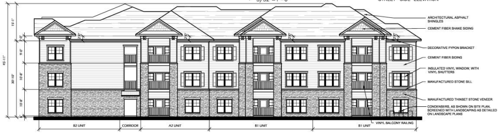
2 BUILDING TWO - EAST ELEVATION 3/32"=1'-0"
