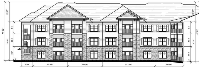
1 BUILDING THREE - EAST COURTYARD ELEVATION 3/32"=1'-0"
