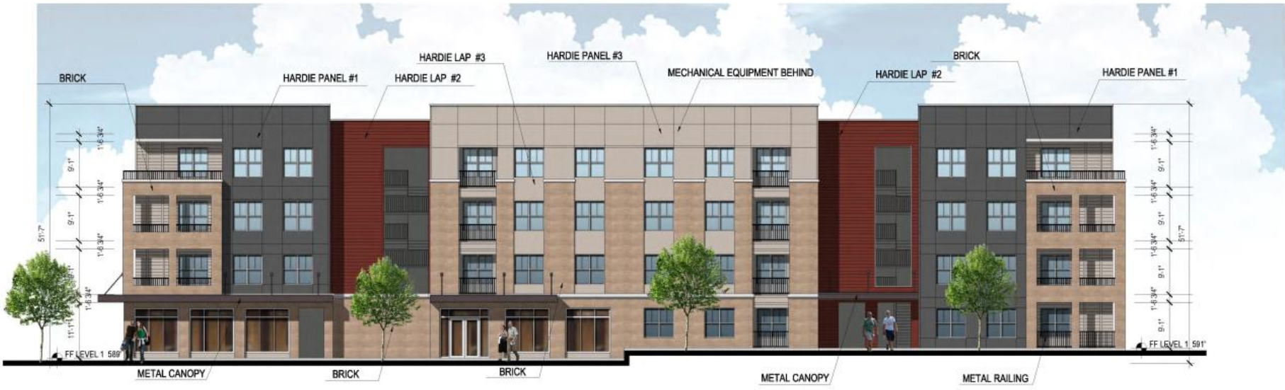
BLDG 2 FRONT ELEVATION
