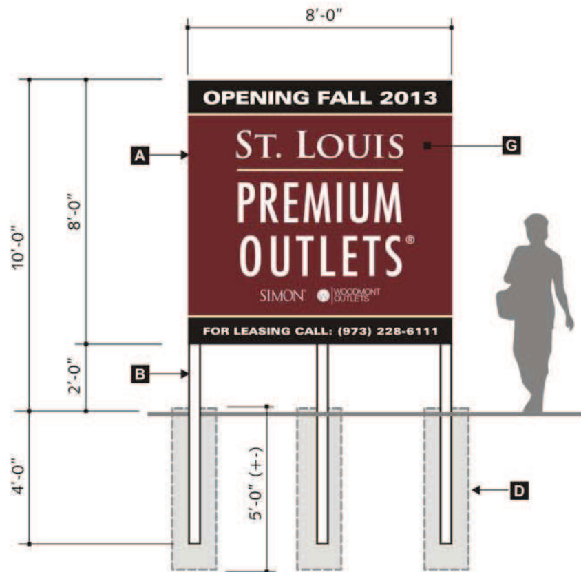
A Front Elevation (T2) Scale: 1/4" = 1'-0"
