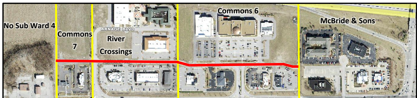
Figure 3—Multi-Development Cross Access Drive
