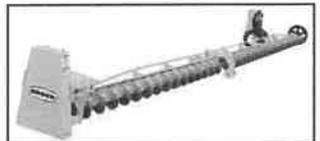
**2000 Series Sweep** – Engineered for heavy farm to light commercial duty. For bin diameters: 30 to 78 feet (9.1 to 23.8 m). Auger diameters: 10 or 12 inches (254 or 305 mm). Capacities range up to 6,500 bushels (165 metric tons) per hour.
