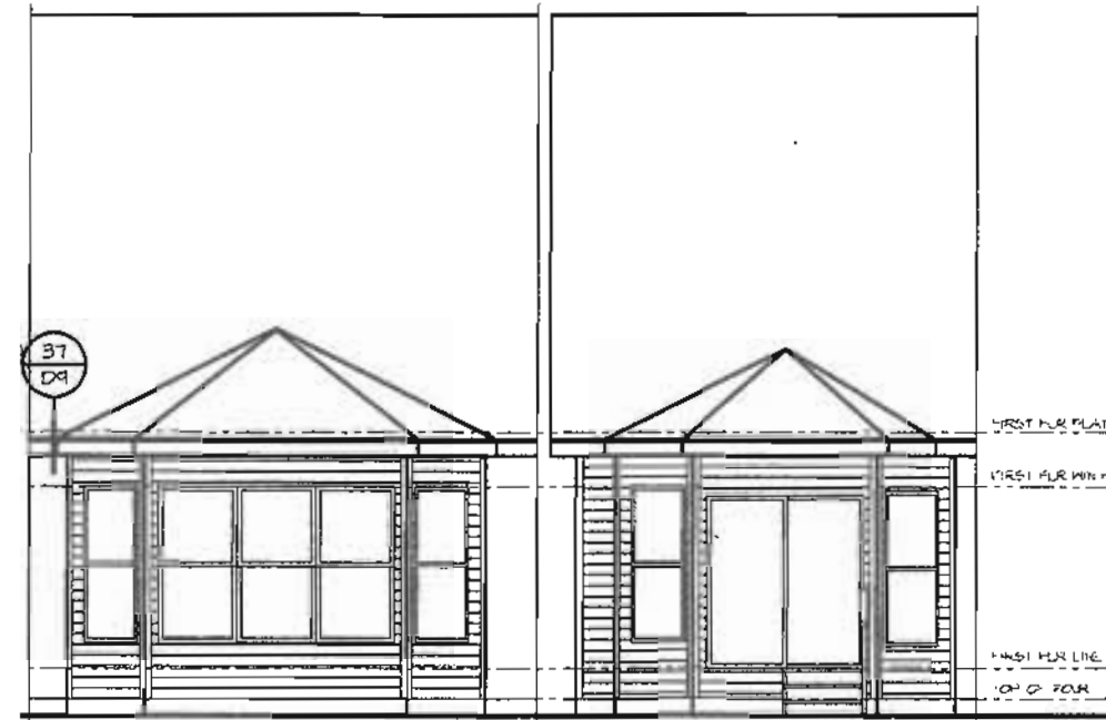
OPT BAY AT BREAKFAST RM REAR ELEV "A" SCALE: 1/8" = 1'-0" (2X SCALE @ 22x34 SHEET)
