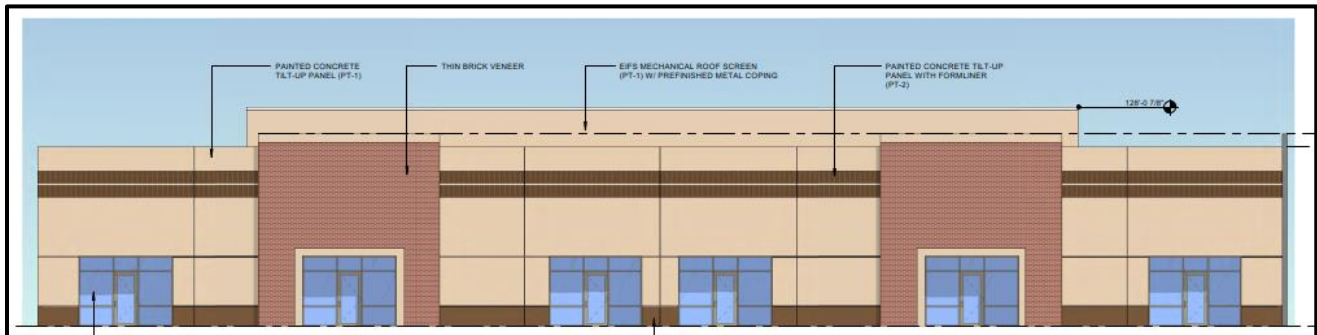
Figure 6: Warehouse/Office Building Front Elevation
