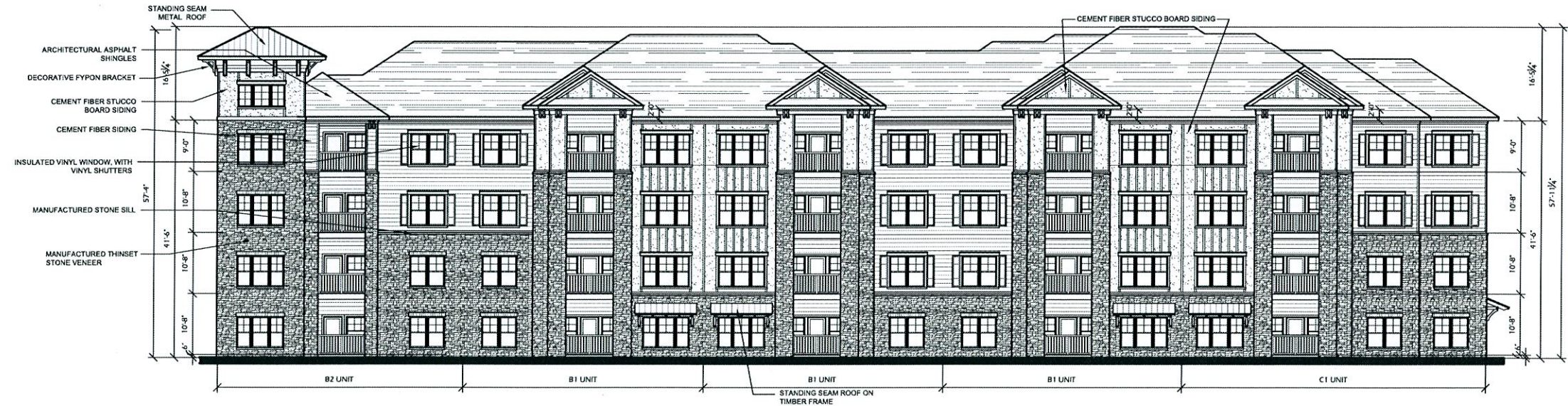
2 BUILDING ONE - EAST ELEVATION 3/32" = 1'-0" STREET-SIDE ELEVATION
