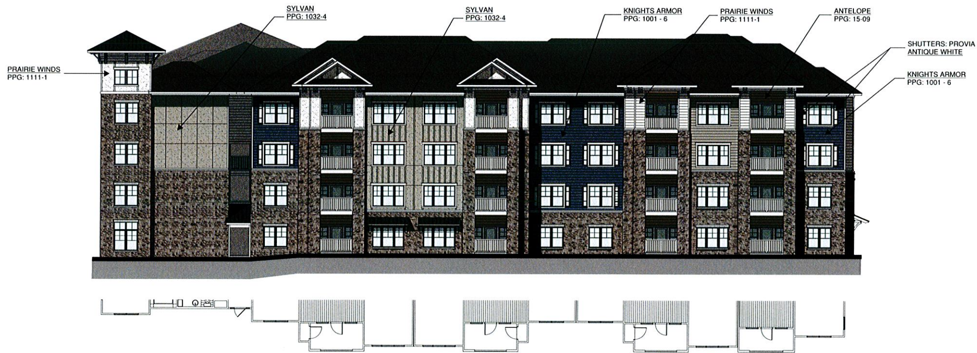
1 BUILDING TWO - EAST ELEVATION 3/32" = 1'-0"
