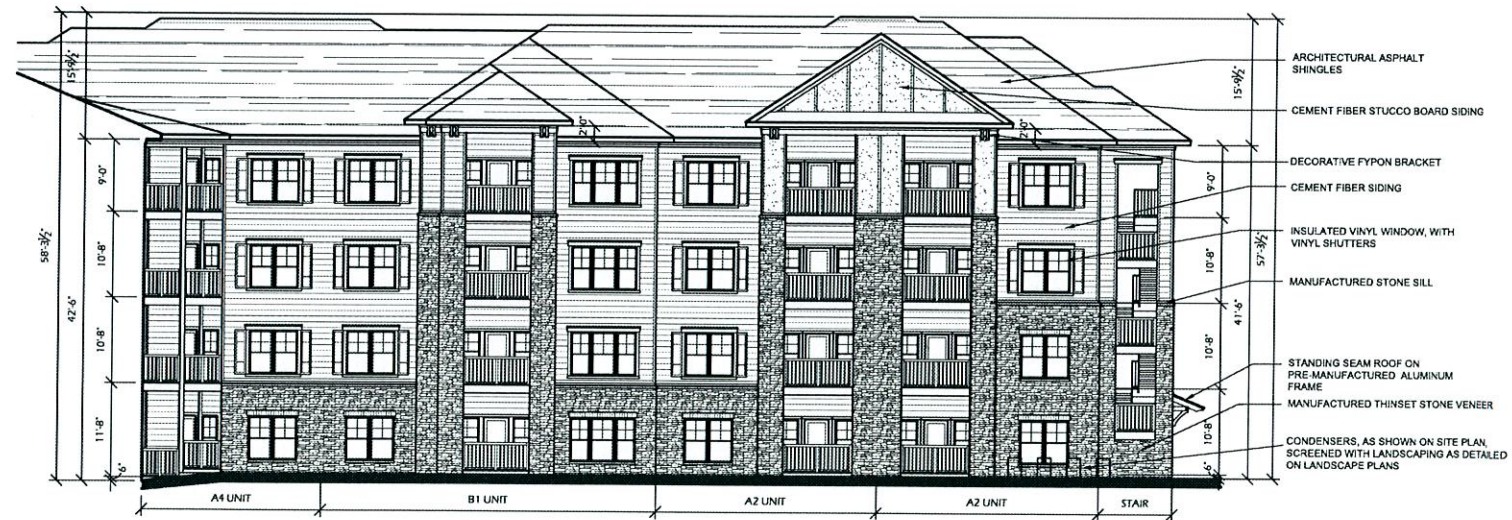
2 BUILDING TWO - WEST COURTYARD ELEVATION 3/32"=1'-0"
