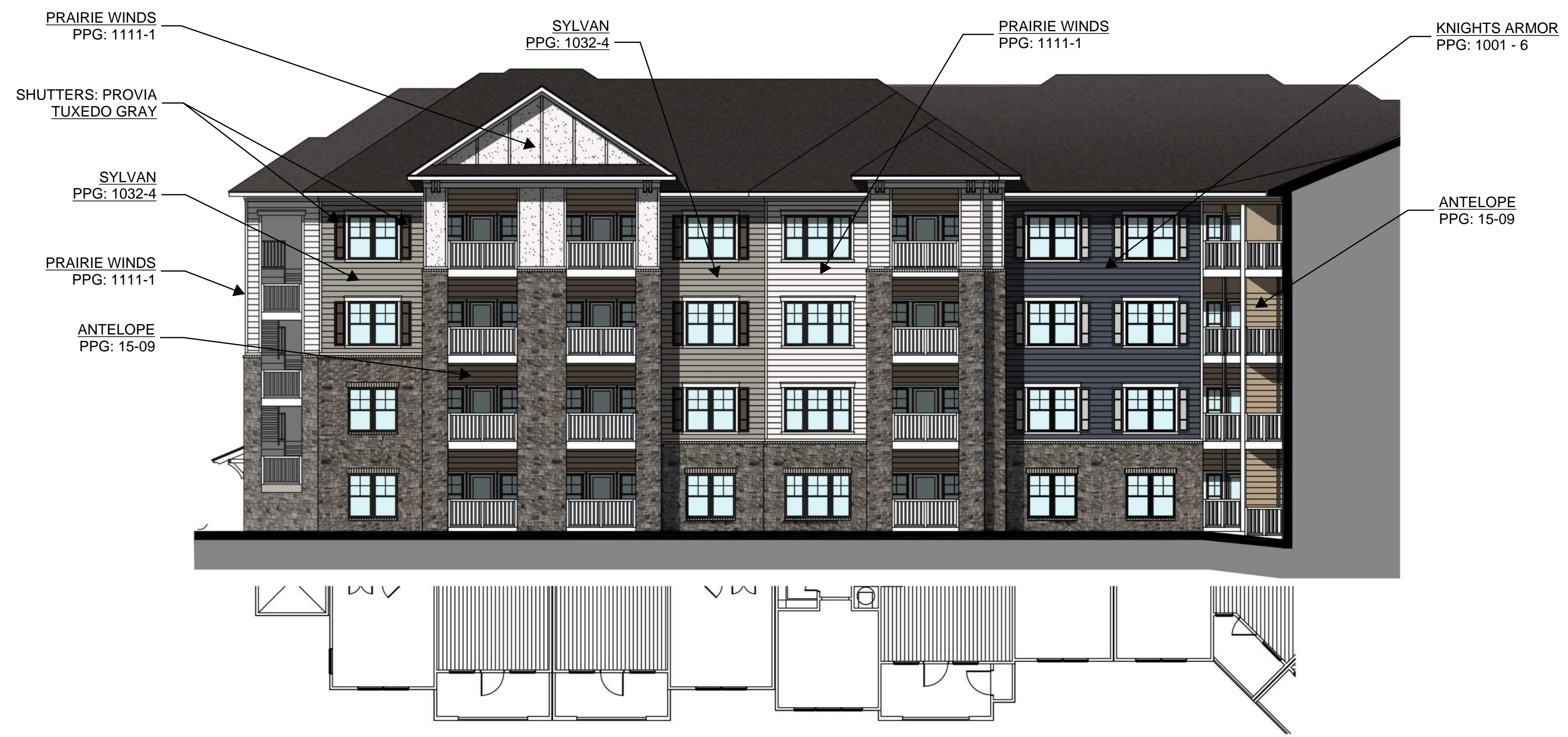
1 BUILDING TWO - EAST COURTYARD ELEVATION 3/32" = 1'-0" 0' 4' 8' 16' 32'
